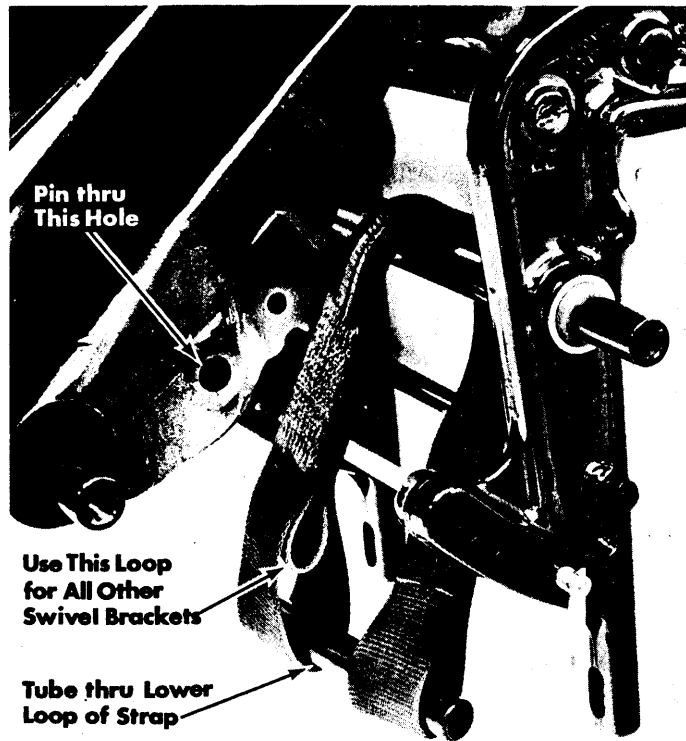
Figure 2. New Design Swivel Bracket for 1975 Merc 850-1150-1500
