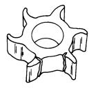
4 - 45 Sec. 2000 RPM All Vanes Broken and Charred - Both Sealing Rings Charred
