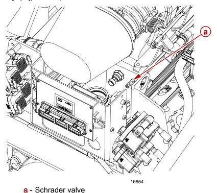
3. Disconnect the pump electrical harness at the fuel pump harness connector.
