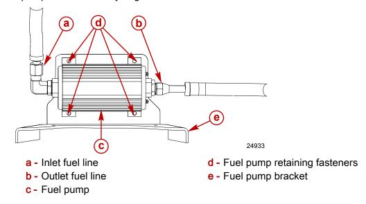
6. Remove both the straight and 90° fittings from the pump and retain for installation.
