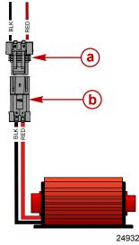
a - Engine harness connector to fuel pump
